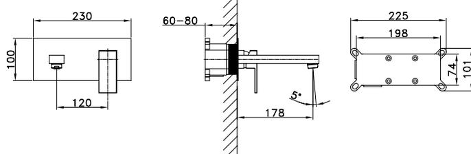
Technical drawing showing dimensions for the faucet handle and its installation into the wall:
